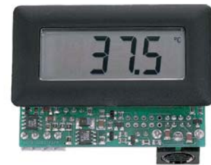
12 Bit (±1999 counts) Data Logger
