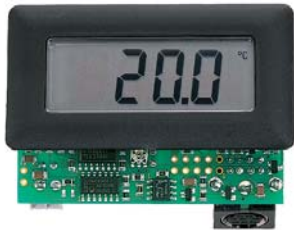
8 Bit (256 steps) Data Logger
